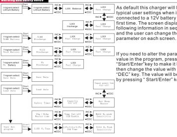
As default this charger will be set to typical user settings when it is connected to a 12V battery for the first time. The screen displays the following information in sequence and the user can change the
